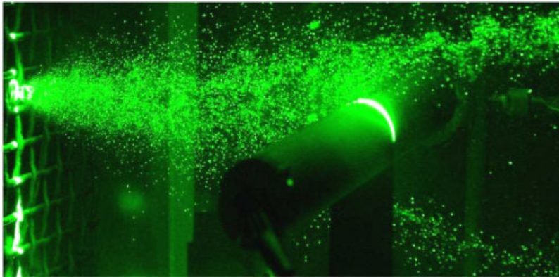
Figure 10. View of the injected water spray over the unheated cylinder of experiment [37]. Effective cone angle is 20^\circ .
