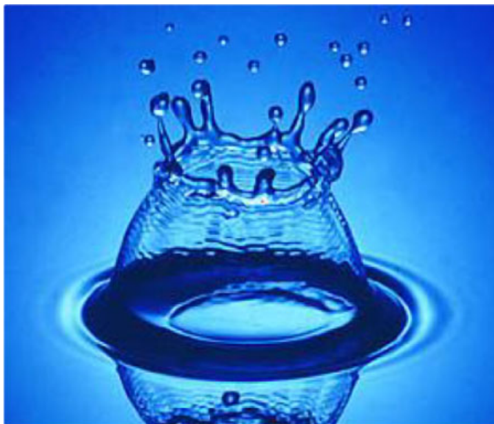
Figure 1. Formation of satellite droplets around the ‘crown’ rim [6] at low-speed impact. Circumferential length of a ring with respect to the rim diameter is l = \pi D_{\text{max}} = 39d_{\text{rim}} . Applying the Rayleigh instability ( \lambda = 4.51d_{\text{rim}} ) yields the number of satellite droplets, N = l/\lambda \approx 9 , which seems to be in agreement with the number of satellites in this figure. Printed with the permission of Andrew Davidhazy of Rochester Institute of Technology.
